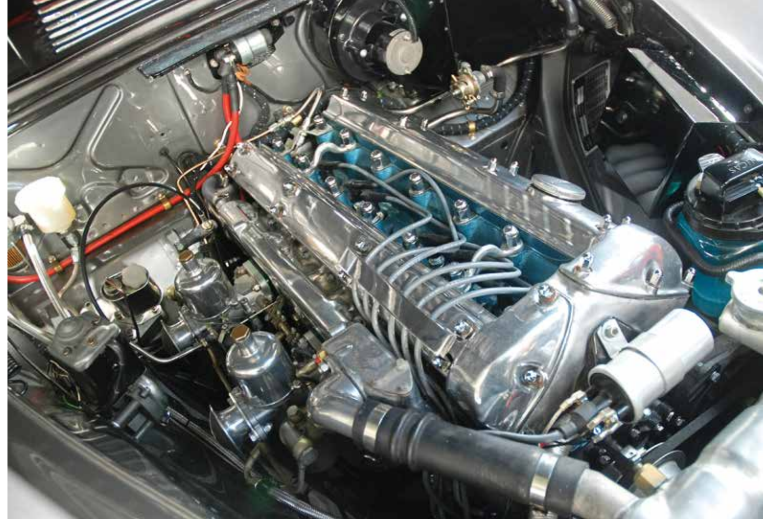
ABOVE: Dash is pure Mk 2, but with luxurious veneer and a Piano Black instrument panel BELOW: Still wearing its B-type 'head', this 3.8-litre engine packs a punch
