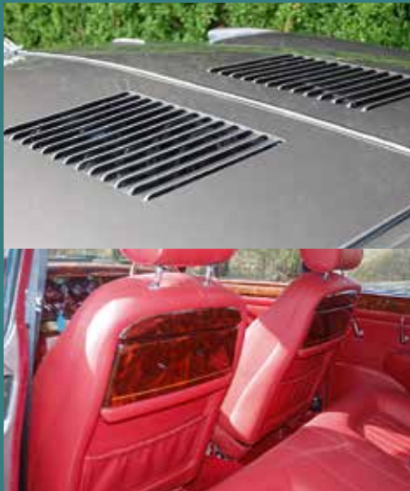
ABOVE LEFT: Aluminium louvred bonnet was fabricated in-house. ABOVE: Seats may be from the X308, but they still have picnic tables in the back. ABOVE RIGHT: The subtle increase in the Coombs-inspired wheelarch flare is almost impossible to see.
